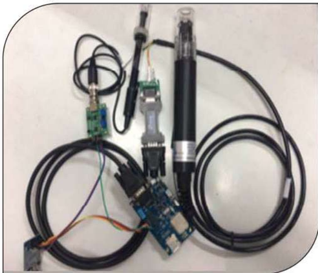
Fig. 4. Sensor measuring DO, Temperature & pH (Courtesy : Huan et al., 2020)
